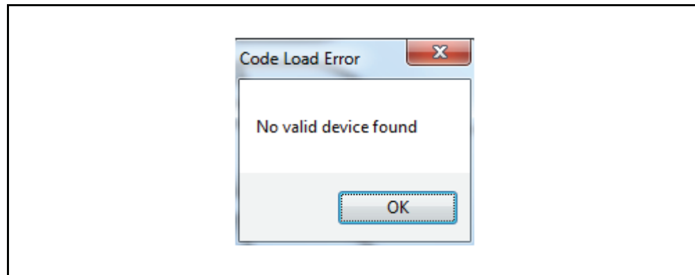
FIGURE 1-9: ERROR MESSAGE IF DEVICE ID IS MISSING IN THE COMMENTS OF LOADED CODE
