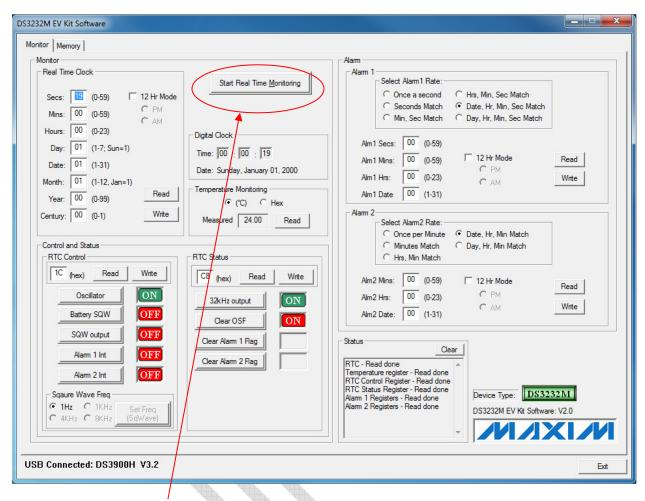
Depressing the 'Start Real Time Monitoring' button puts the application into a continuous-read loop, updating the real-time, alarm, status, control, and temperature sensor register contents. Once started, this button renames itself to 'Stop Real Time Monitoring', and the green LED (D2) on the DS3900H2 will blink red upon each component read.
