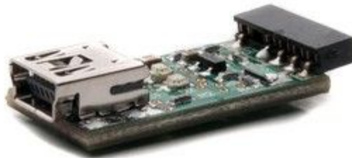
Figure 6.3: A debug module connects to your target system
