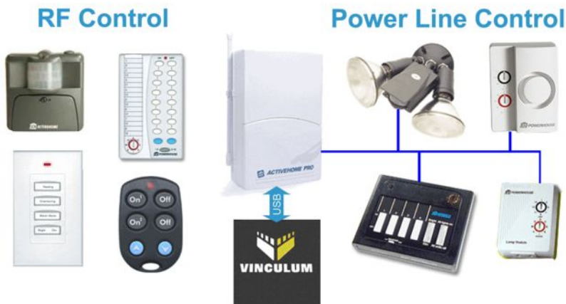
Figure 10.9: X10 system with many real-world inputs and outputs
