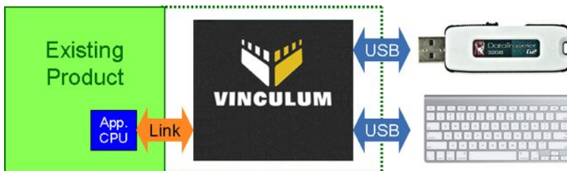
Figure 5.1: Vinculum-I operates as an attached device
