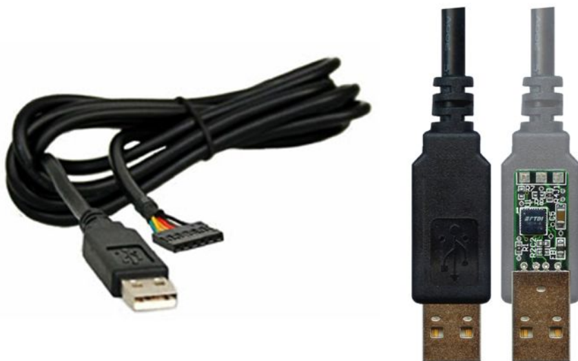
Figure 2.1: The TTL-232R is a USB-to-4BitIO port cable
