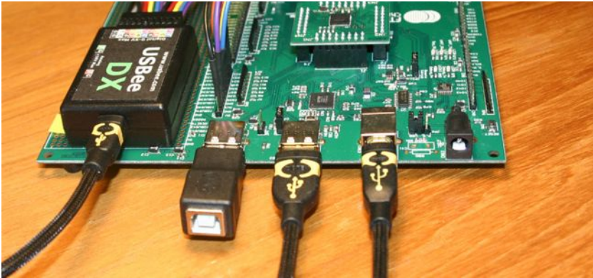
Figure 9.6: USB device development uses a USB gender changer
