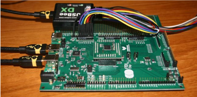
Figure 8.4: Connecting the USBee LA to the V2EvalBoard
