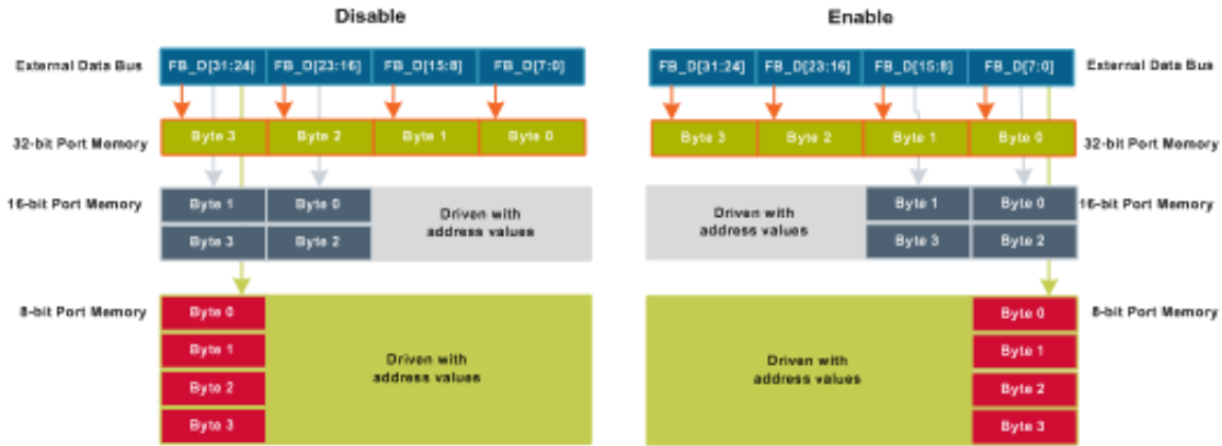
Figure 10-2. Sequential 32-bit transfers, byte lane shift differences
