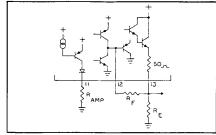
Operational Amplifier Internal Input Circuitry
