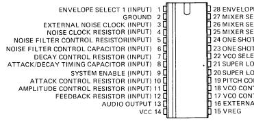
28 ENVELOPE SELECT 2 (INPUT)  $\square$  27 MIXER SELECT C (INPUT) 26 MIXER SELECT A (INPUT) 25 MIXER SELECT B (INPUT) 24 ONE-SHOT CONTROL RESISTOR (INPUT) 23 ONE-SHOT CONTROL CAPACITOR (INPUT) 22 VCO SELECT (INPUT) 21 SUPER LOW FREQUENCY OSC. CONTROL CAP. (INPUT) 20 SUPER LOW FREQUENCY OSC. CONTROL RES. (INPUT) 19 PITCH CONTROL (INPUT) 18 VCO CONTROL RESISTOR (INPUT) 17 VCO CONTROL CAPACITOR (INPUT) 16 EXTERNAL VCO CONTROL (INPUT)
