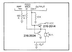
If the amplitude of the sound output is to be varied for particular sounds, the resistance RAMP can be varied by logic control lines. This can be done (as described earlier) by using the logic control line to switch a logic gate that will put a resistor in parallel with RAMP.
