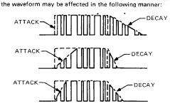
Figure 5: Examples of Varying Degrees of Attack and Decay on a Waveform
