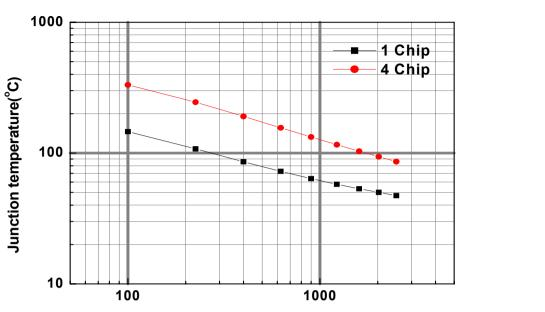
Heat sink area(mm<sup>2</sup>) (1.5t Al Heat sink)
