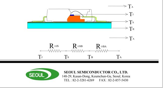
$R\Theta$  of Z-Power LED is calculated from junction to metal PCB bottom.
