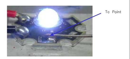
$\Delta Tc$  in graph means difference Temperature between On and Off,
