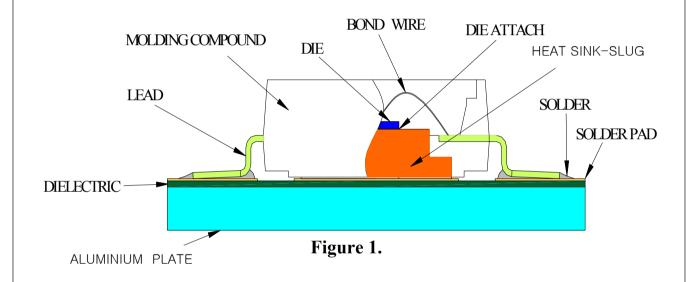
Z-power LED is composed by mounted chip on bottom of heat sink slug and solder pad of AI-PCB. Heat sink slug is composed the materials as copper that has high thermal conductivity.
